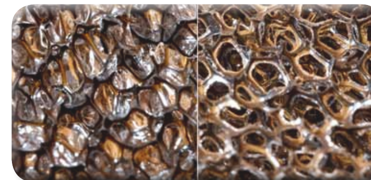
Foam before and after reticulation
